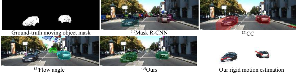
Figure 5: Comparison on KITTI-SF, image 137. The prefix of each method indicates the test-time inputs: (1) Single frame. (2) Multi-frame with appearance features. (3) Multi-frame without appearance. Our best appearance-based segmentation baseline, (1) Mask R-CNN [20] detects all the moving vehicles, but also reports parked cars in the background. (2) CC [39] correctly detects moving cars but also reports the edge of the road as moving objects. (3) Geometric segmentation algorithm [5, 58] fails on the approaching car due to the colinear motion ambiguity, and reports false positives at the background due to the noisy flow estimation. In contrast, (3) our method correctly segments both the moving vehicles and the rigid background. Rigid motions are estimated within each mask and applied to depth and scene flow estimation.
