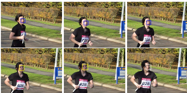
Figure 11. Face tracking using an NCC-FF-MS cascade. NCC (blue) is used initially, switching to FF (yellow) when a strong shadow is cast on the face. Subsequently the tracker switches to mean-shift (white).
