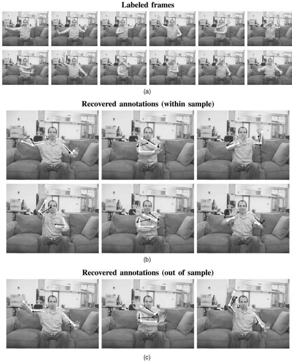
Fig. 8. (a) Twelve frames were annotated with the joint positions of the subject in a 1,500 frame video sequence. (b) The recovered positions of the hands and elbows for the unlabeled frames are plotted in white. The output of fully supervised nonlinear regression using only the 12 labeled frames and no unlabeled frames is plotted in black. Using unlabeled data improves tracking significantly. (c) Recovered joint positions for frames that were not in the training set. The resulting mapping generalizes to as-yet unseen images.
