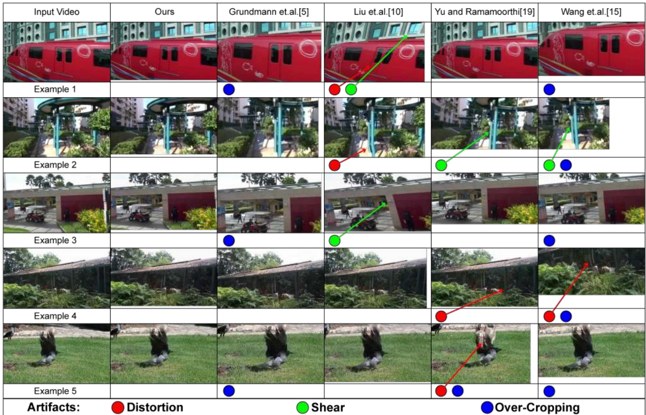
Figure 13. The visual comparison of Grundmann et.al.[5], Liu et.al.[10], Yu and Ramamoorthi[19], Wang et.al.[15] and our method. The artifacts are noted below the video stills and pointed out by arrows. To avoid introducing extra distortion, all the video stills are scaled while keeping the original aspect ratio.
