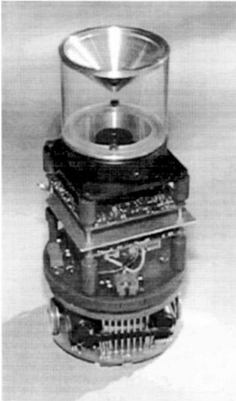
Figure 2. Khepera™ robot with camera module and custom made conical mirror, which permits sampling of the environment over 360°, in a range of \pm 10^\circ about the horizon.
