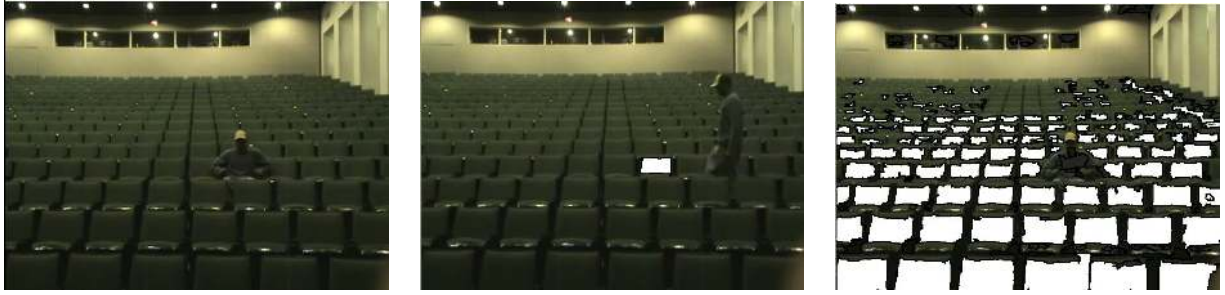
(a) Example 1: A person is tracked in a theater as they walk in from the left and sit down in a chair. This sitting down action is detected by the activity recognizer which triggers the search for “chair” objects.
