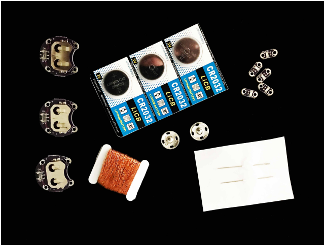
Figure 3: The supplies sent to the participants with the sampler: 3 battery holders, 3 batteries, conductive thread, 2 snaps, 5 LEDs, 2 sewing needles.
