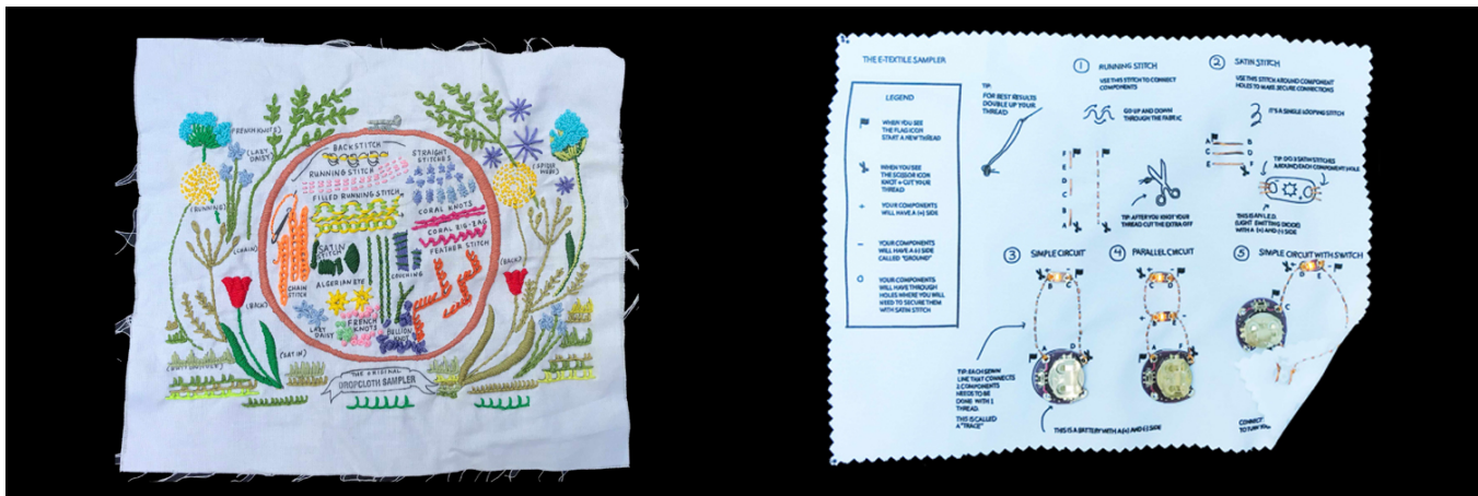
Figure 1: (left) A modern stitch sampler designed by Dropcloth Samplers used for learning embroidery techniques; (right) the e-textile sampler designed for this study for learning stitches and circuit basics.
