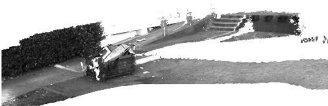
Fig. 5. Globally aligned point cloud model for a dataset composed of approximately 1600 stereo frames.
