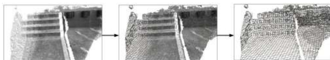
Fig. 6. Point Cloud model simplification using polygonal fitting. From left to right: overlapping aligned point cloud views, combination PCD model and polygonal model, and the resulting polygonal model.
