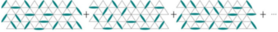
Fig. 2.9 The nearest-neighbor RVB state is the superposition of all possible configurations of nearest-neighbor singlets
