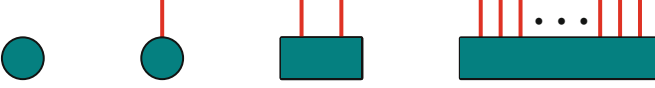
Fig. 2.1 From left to right, the graphic representations of a scalar, vector, matrix, and tensor
