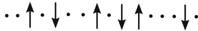
Fig. 2.5 One possible configuration of the sparse anti-ferromagnetic ordered state. A dot represents the S = 0 state. Without looking at all the S = 0 states, the spins are arranged in the anti-ferromagnetic way
