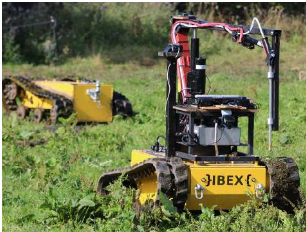
Fig. 1 Example of an autonomous small robot for agriculture (agribot). This agribot weighs 250 kg and precision spray weeds on hill farms. (Photo: Ibex Automation Ltd.)
