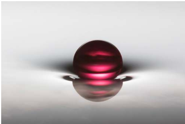
FIG. 1. An ethanol drop with red dye levitates in the Leidenfrost state over a pool of silicone oil V20. The drop radius is R = 1.2 mm and the pool is at T_p = 79^\circ\text{C} while the boiling point of ethanol is T_{\text{sat}} = 78^\circ\text{C} . (Image credit: Florence Cavagnon).
