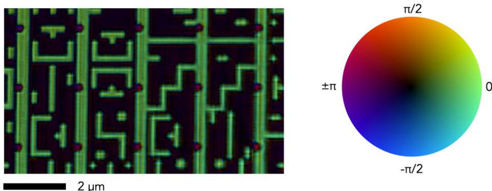
Figure 4. Reconstructed complex amplitude map of a sample with a buried array of carbon pillars with 200 nm diameter and 3.5 nm height.
