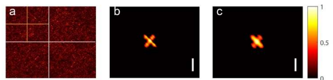
Fig. 5. Image reconstructions from a section of the raw speckle image. (a) The raw speckle image captured by the camera. (b) The reconstructed object calculated from the top left 1/4 section of the speckle image. (c) The reconstructed object image calculated from 1/16 section of the speckle image. Scale bar is 2mm, same as the object size.
