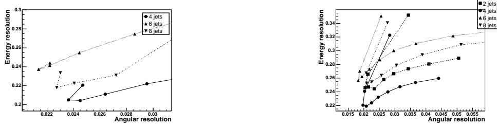
Fig. 45: Relative energy resolution versus angular resolution ( \Delta R distance between jet and quark) for the IC algorithm (left) and k_T algorithm (right). The markers of the same type represent the seven different IC cone radii (0.2-0.8) or the ten R-parameter values (0.1-1). The values on the top left are the ones with the smallest cone radii or R-parameter values, respectively. The energy resolution is defined as the RMS divided by the mean value of the E^{jet}/E^{quark} distribution, and the angular resolution is defined by the width of a gaussian fit to the symmetrized \Delta R distribution. For this plot, the two quark-jet pairs with the worst matching (only the worst one in the case of two jets) have been removed to reduce the effect of radiation.
