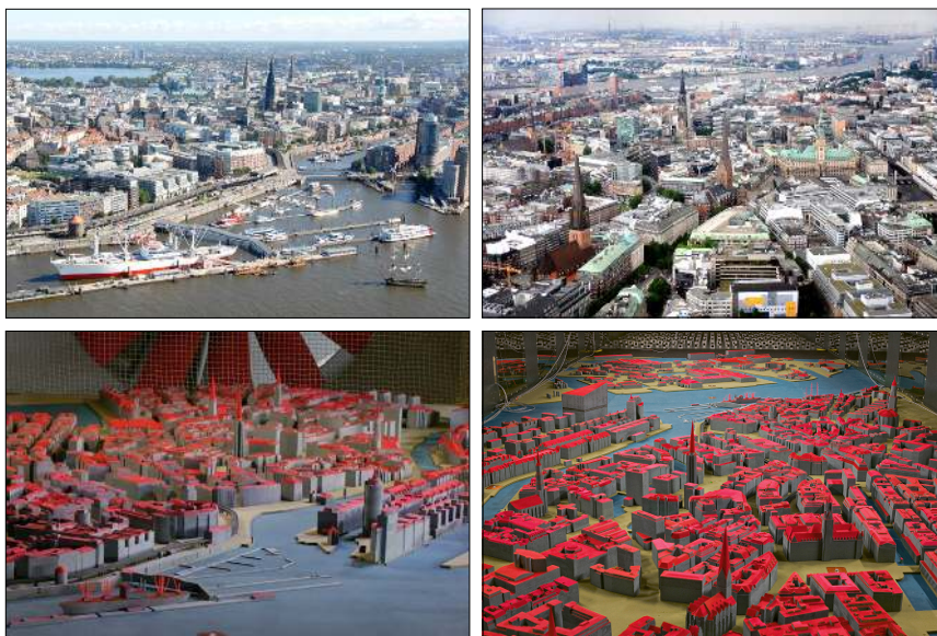
Fig. 4: Aerial photographs of the central part of the Hamburg domain together with the representation in the wind-tunnel model. Left: view from the south-west towards the inner city area. Right: view from the north-east towards the industrial harbour.
