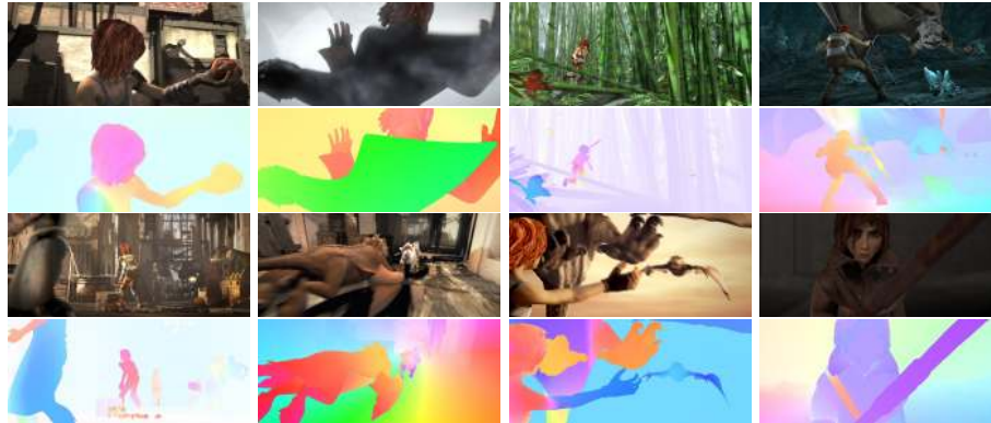
Fig. 1. Examples. Example frames from 8 of the 35 scenes contained in our dataset. The ground truth optical flow is shown below the corresponding rendered frame. Color coding as in [1].
