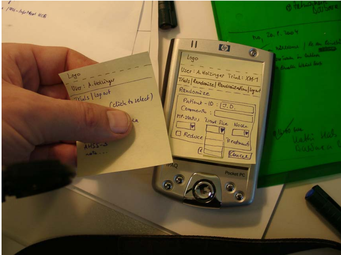
Fig. 2 Paper Mock-ups proved to be efficient within the development of the Randomizer
