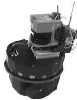
(d) Hilare platform with a manipulator (LAAS-CNRS) Rectangular differential drive, SICK Laser
