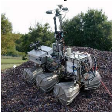
(e) Lama platform (LAAS-CNRS) Rectangular differential drive, stereo vision
