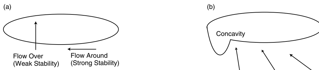
Figure 2. Schematic diagram of Alpine-scale orographic flow modification illustrating (a) the importance of weak stability enabling the depicted southerly flow to surmount the tall Alpine barrier instead of flowing around (to the west in the Northern Hemisphere), and (b) the effects of Alpine shape in directing southerly flow towards the concavity.
