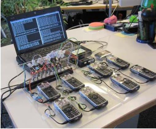
Figure 3: Experimental setup: Motorola C1XX phones with custom firmware, GPS receivers, and a laptop for serial communication.
