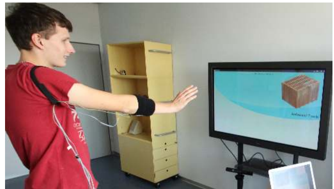
Figure 1: Free-hand interaction with haptic feedback: A user receives haptic feedback when approaching an object shown on the screen.
