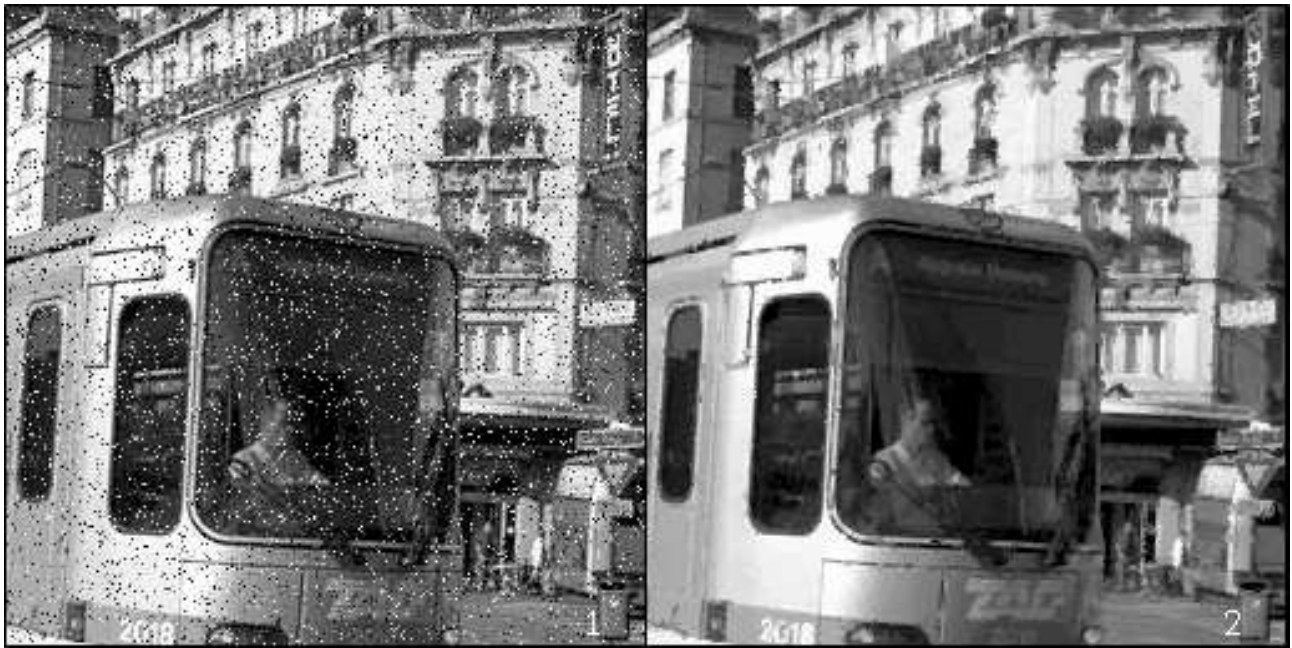
Figure 4: Left – Noisy image (impulse noise, frequency = 10%) Right – Occlusion detection is performed with the grain filter (see [6]); occlusions are non-invariant sets. Disocclusion is then achieved with our level lines based algorithm.
