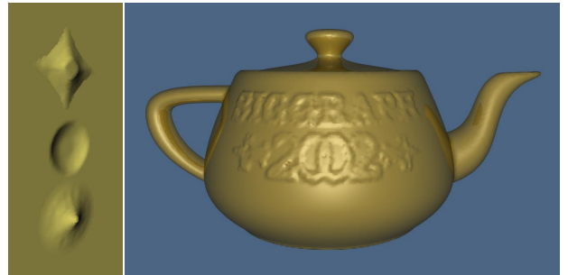
Figure 8: Left: Three types of single point attractions/repulsions using different ROI primitives and \gamma values. Right: Utah teapot embossed with 7862 points sampling the “SIGGRAPH 2002” logo.
