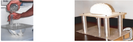
Fig. 3. Elastic PVA-C brain phantom: (a) liquid stage (b) final result after freezing and thawing.
