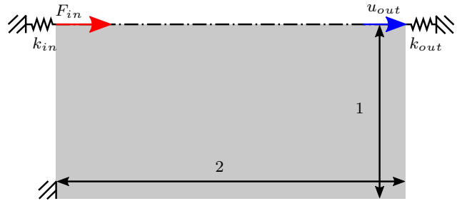
Fig. 26 Force inverter design problem. The material has stiffness E = 1 and \nu = 0.3 and the input and output springs are set to k = 0.1 . The input force is set to F = 1 .
