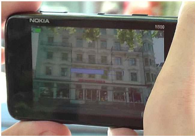
Fig. 1 A cell phone picture is taken to localize the user and to retrieve point-of-interest information from the database. We assume to know the camera's focal length and that we can identify the vertical and horizontal facade direction by means of vanishing points to allow for rotation invariant recognition
