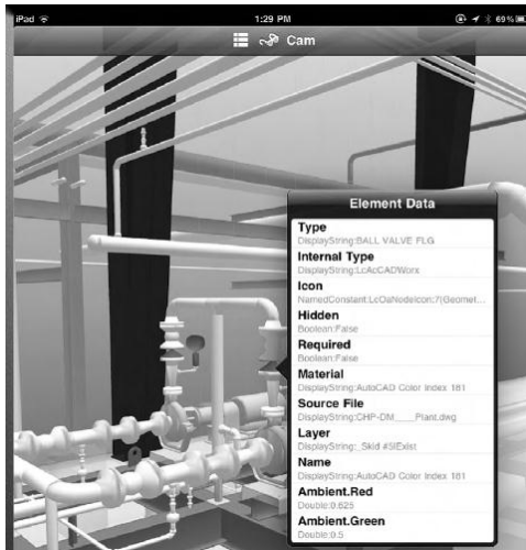
FIG. 11: Field BIM ties BIM models to the field for data and document exchange (Source: Vela Systems, 2011).
