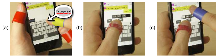
Figure 17: Smartphone selectors: (a) middle correcting a word; (b) thumb used as a selector and showing the crib sheet; (c) index triggering copy
