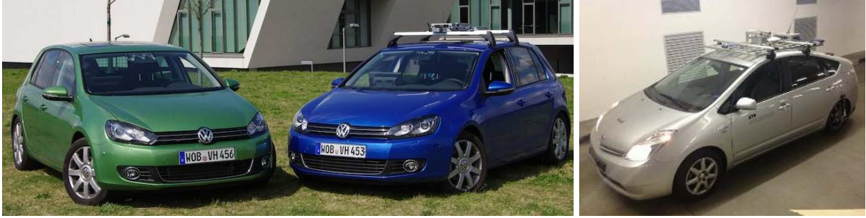
(a) The Volkswagen Golf platforms. The cameras are integrated into the car body. (b) The Toyota Prius platform. The cameras are mounted on the roof rack.
