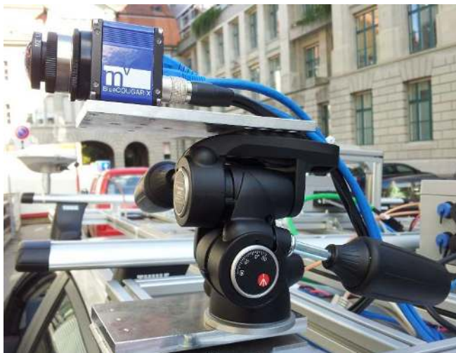
Figure 23: The left camera is mounted on a three-way tripod head, which in turn, is mounted on a sliding plate. This sliding plate is attached to the car roof via screws.
