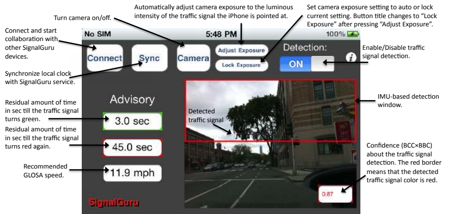
Fig. 4: SignalGuru service screenshot. GLOSA advisory has also been included in the same iPhone application. Audio advisory can complement the visual advisory to alleviate driver distraction.
