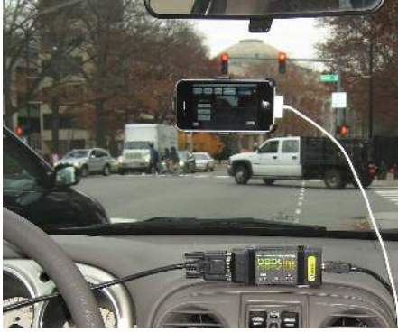
Fig. 3: SignalGuru-enabled iPhone mounted on the windshield. The OBD-LINK device used to measure fuel consumption is also shown.
