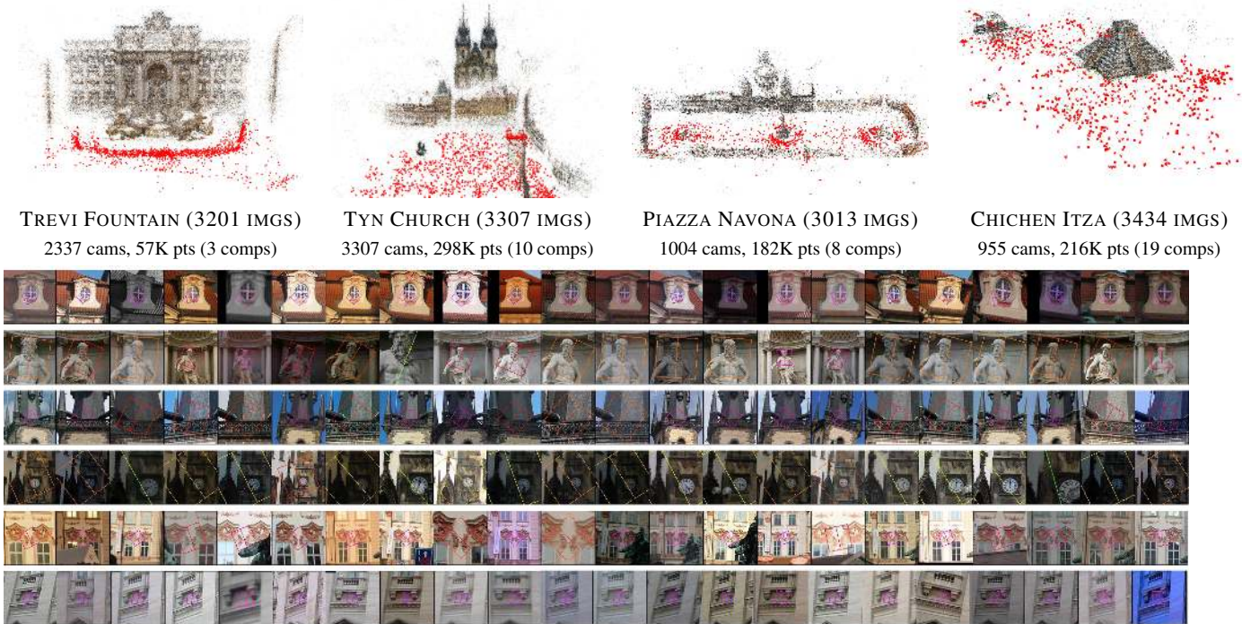
Figure 1: [TOP]: Examples of SfM reconstructions from LANDMARK-620 our Internet photo collection dataset (the largest component is shown and the number of cameras and 3D points are listed). [BOTTOM]: Six out of approx. 8 million tracks i.e. sets of matching keypoints recovered from running SfM on LANDMARK-620 (patches are visualized at their original scales).
