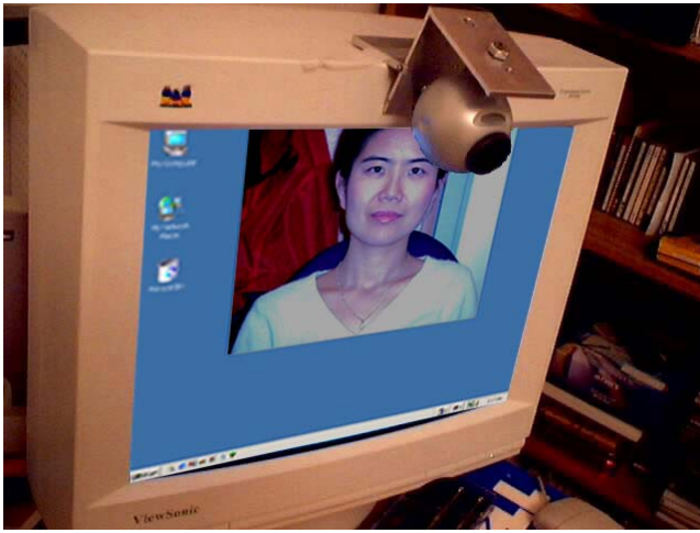
Figure 7. Desktop videoconference prototype. We constructed a mechanical camera holder so that an inexpensive desktop conferencing system can support eye contact.
