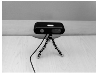
Fig. 1. PrimeSense Reference Design USB plug-and-play device
