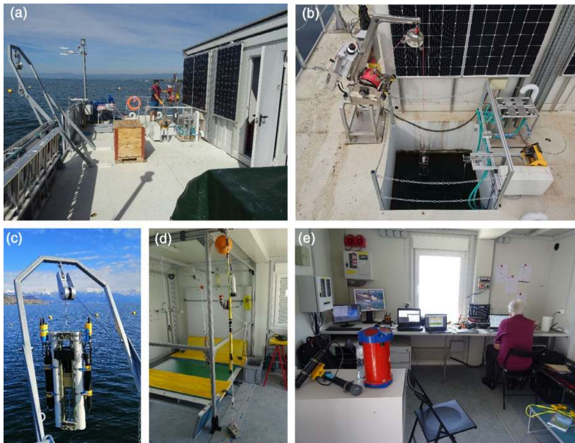
FIGURE 2 LéXPLORE elements (from top left to bottom right): (a) outdoor work area, (b) outdoor moonpool with electric crane (left) and pump system (right), (c) Wirewalker deployment using an A-frame, (d) partially covered indoor moonpool, and (e) office work area
