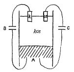
and chlorine ions in the solution. The alloys are in electrical contact with the mercury, and electromotive forces can be inserted in the circuits thus formed at B and C. The potential difference between the solution and the mercury can be increased by removing from the solution small amounts of ionic mercury and chlorine by means of the circuit C.
