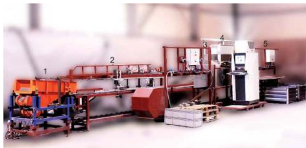
Fig. 6 Prototype sorting machine for refractories with integrated LIBS unit (material flow from left to right). (1) feeding, (2) singularisation, (3) 3D-camera, (4) LIBS unit, (5) sorting. Photo: Fraunhofer ILT at the facilities of Orbix, Genk, Belgium.
