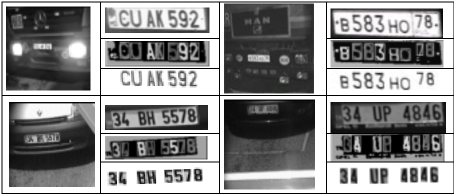
Fig. 5. Experimental results for five test images which include various sizes and forms of license plates.
