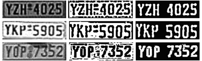
Fig. 10. Successful segmentation of characters following the SCW method. (Left column) Original segmented plate, (middle column) SCW result, and (right column) character segmentation after negation and height and orientation measurements.
