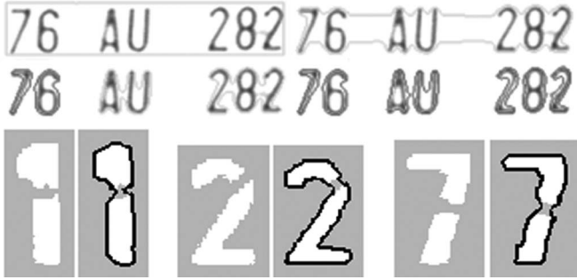
Fig. 8. (Top) Segmentation sequence. (Bottom) Merging broken characters.
