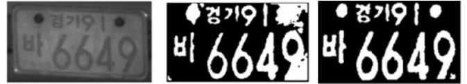
Fig. 9. Binarization results from left to right: noisy LP image, global threshold, and adaptive threshold in [59].
