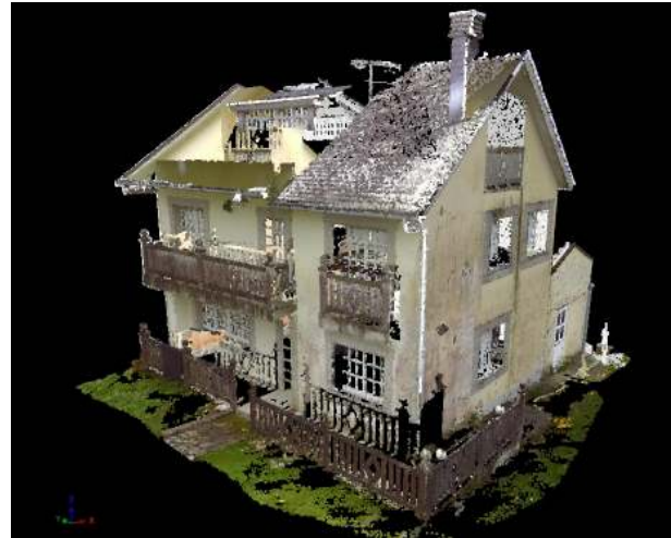
Figure 6. Reference point cloud, measured with the terrestrial laser scanner FARO Focus 3D X330.
