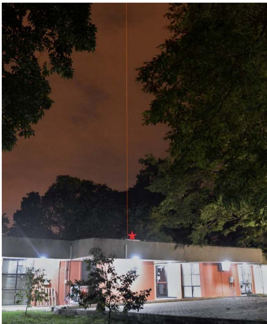
Figure 6. Picture showing the dual-beam Na/K lidar located at São José dos Campos, Brazil. The vertical orange beam is at 589 nm for Na scattering and the infrared one at 770 nm for K scattering. This last is not visible in the photo, but the red star indicates the beam position. Liu Zhengkuan took the original photo.
