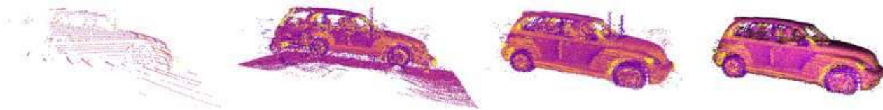
Figure 4: From left to right: Individual sweep, Accumulated cloud, Symmetry completion, outlier removal and surfel meshing
