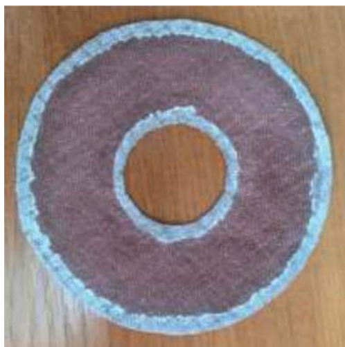
Figure 4. Same woven fabric with plasma copper coating.
