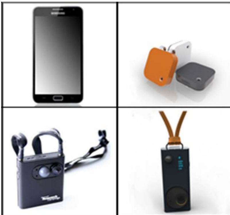
Figure 1. Examples of mobile devices for lifelogging. Top: Smartphone (left), and Memoto wearable camera (right). Bottom: SenseCam (left) and Autographer (right) wearable cameras.
