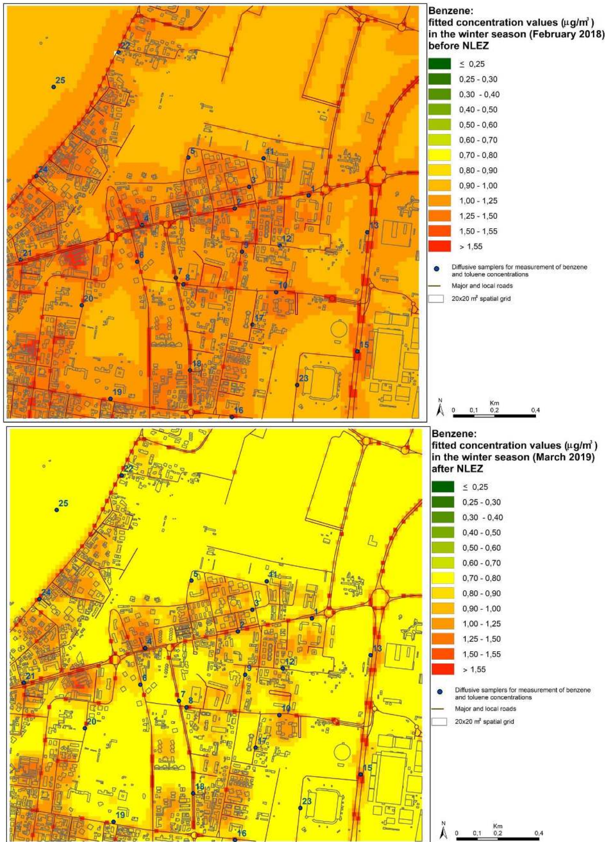
Figure 15: Benzene winter concentration levels ( \mu\text{g}/\text{m}^3 ) estimated from GAM models before (left) and after (right) Noise LEZ implementation
