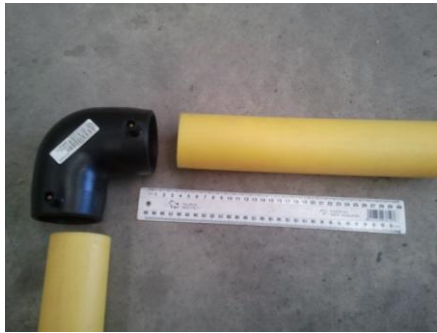
Figure 14: Example of MDPE electrofusion joint for the Contact Energy pipes
