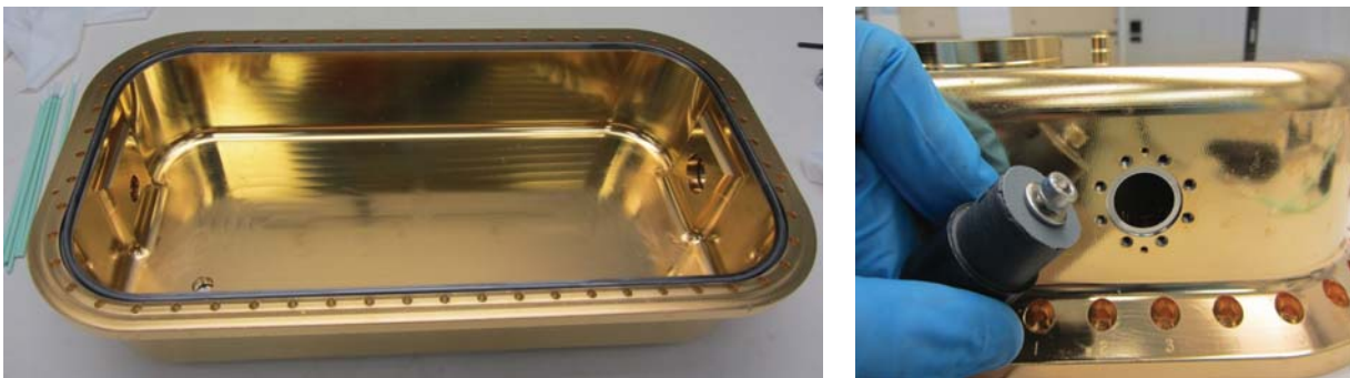
Figure 13 Left: Enclosure cover showing the custom rectangular c-seal. Right: Polishing tool and the polished window interface for the round c-seal.
