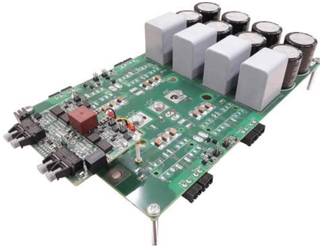
FIG. 5. Test board for the characterization of semiconductor modules and/or TO-packaged discrete devices.
