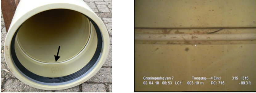
Figure 3.1: Left: image of the interior of a 315 mm PVC joint. The gap is signaled with an arrow. Right: underwater image of the interior of the same PVC joint obtained with CCTV. Please note the difference between this joint and the one presented in Figure 2.2: in this situation the ring separating both joints (white) was molded with the joint and is not a stand-alone piece.
