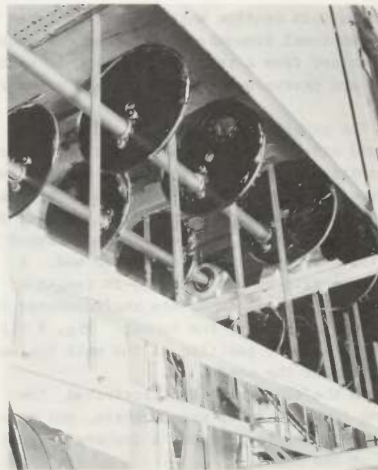
Fig. 4 A view of the springs and cams used to constrain the tunnel wall into a sinusoidal shape
