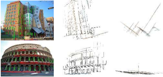
Figure 11. Typical behavior of the line reconstruction algorithm in non-Manhattan scenes. In the first row, MIT Stata center is approximated with Manhattan 3D lines. In the second row, the curved surface of the Colosseum is approximated by a single plane.
