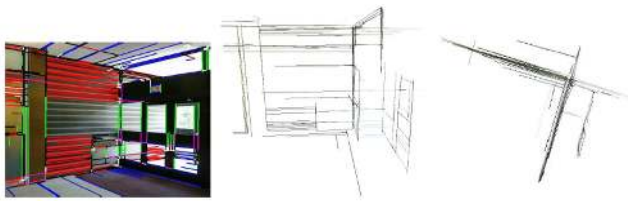
Figure 12. Left: We show an image of an indoor scene with two orthogonal walls. In the middle and right, we show two different perspectives of the line reconstruction. Note that the line reconstruction recovers the second door behind the right wall. Understanding such structures would be challenging for many existing techniques. [Best viewed by zooming]
