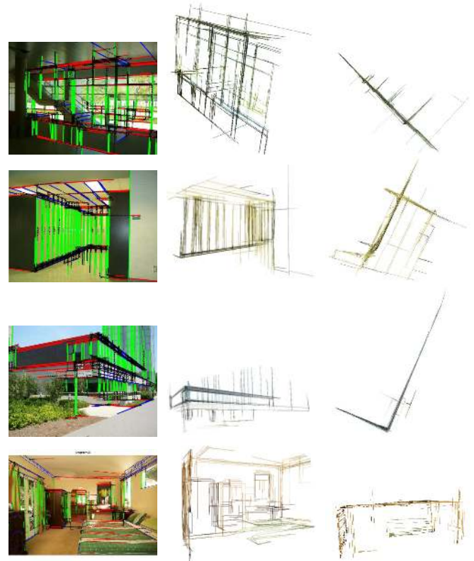
Figure 10. Failure cases in the line reconstruction. In the first row, missing lines along the z direction led to the collapse of the two parallel planes to a single plane. In the second row, spurious lines from the reflections on the shiny floor are mistaken for vertical structure in the scene. In the third row, missing horizontal lines on the background building deprives the LP of evidence that it is a separate structure. In the last row, incorrect focal length estimation using the vanishing points led to smaller estimates for the depth parameters.
