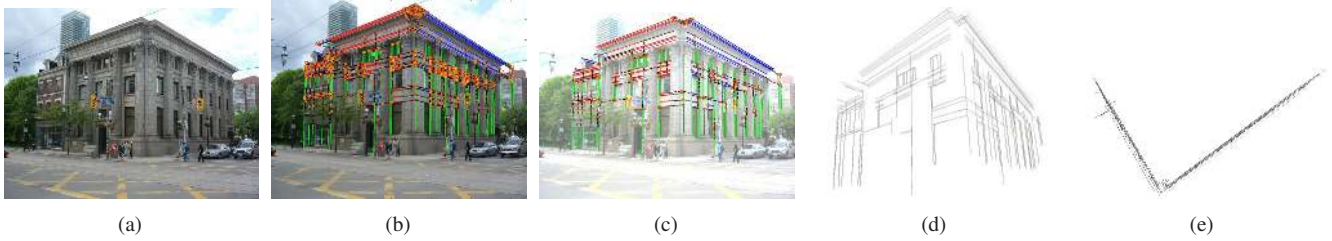
Figure 5. The various stages of our automatic single view line reconstruction algorithm. (a) Given an input image, we extract lines, compute vanishing points and cluster the lines according to three principal orientations. In (b), we show the intersections of the Manhattan lines in the constraint graph. We solve the LP and use the solution to select a subset of constraints using a minimal spanning tree (MST) algorithm. The selected subset is shown in (c). Using the MST we compute the \lambda_i parameters using a linear system. These depth parameters are sufficient to lift the 2D lines to 3D space in the world coordinate system. Two different perspective views of the reconstructed lines are shown in (d) and (e).
